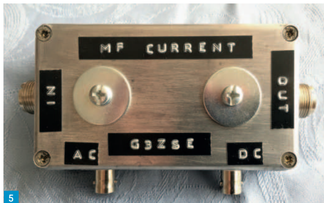
Fig. 5: RF ammeter – boxed. Fig. 6: RF ammeter – inside. Fig. 7: RF ammeter display. Fig. 8: Complete Tx/Rx setup.
